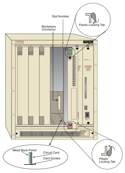
Figure 3-1 Installing an Interface Module
